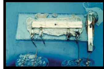
First working integrated circuit on germanium – Texas Instruments, 1958
